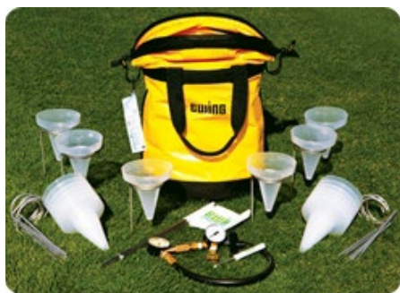
Irrigation performance testing kit including pressure gauge, catchment cups, anemometer, and marking flags to be used by a certified landscape irrigation auditor.
